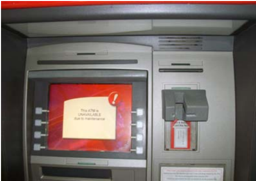
2. Close up of card reader attachment over card slot
