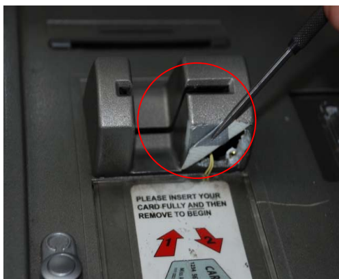
2. The damaged Card reader
